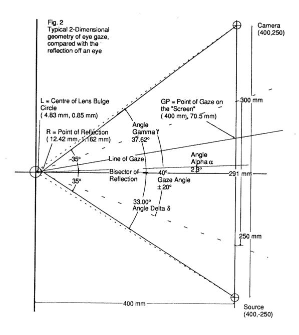
The dimensions of the eye are entered, as are the coordinates in three dimensional space of the "screen" (in the x,z plane) that the subject is looking at and the locations of one IR source and one camera. The source and the camera may be place in any position, independent from each other in the same x,z plane as the screen.
