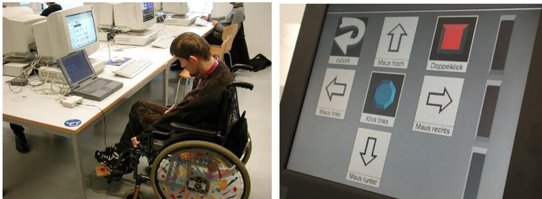
Fig. 10: Wheelchair-using IT student at Vienna University of Technology (left picture) Photo taken in one of the Internet rooms of TU Wien. The student is using AUTONOMY system (right picture) for writing Modula-2 source code.
