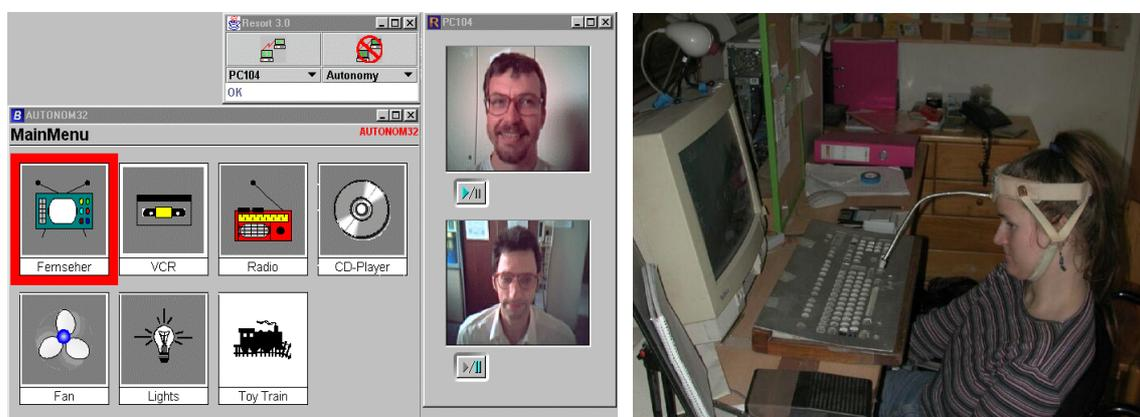
Fig. 9: Screen Shot of client's screen during a RESORT Tele-Help session (left picture). Non speaking head stick user in front of her PC running the commercial version of AUTONOMY for communication in synthetic speech and for environmental control equipped with RESORT tele-help module. The subject is studying biology at Vienna University.
