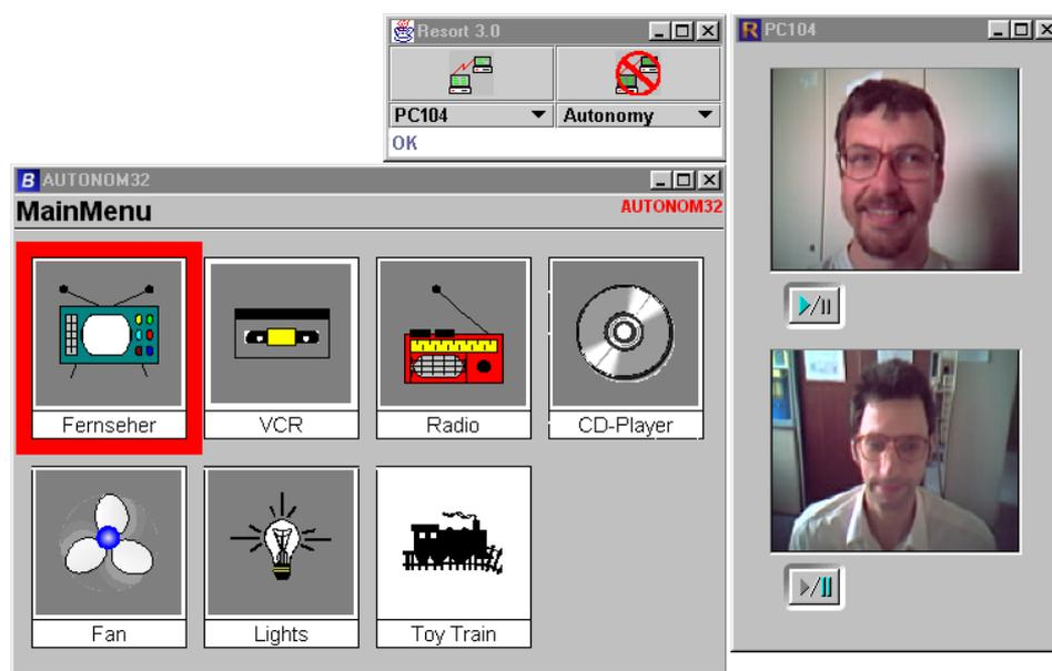
Figure 5. Screen shot of one of the early RESORT prototypes showing a Client PC (left hand ECS / AAC system, above the RESORT controller UI).
