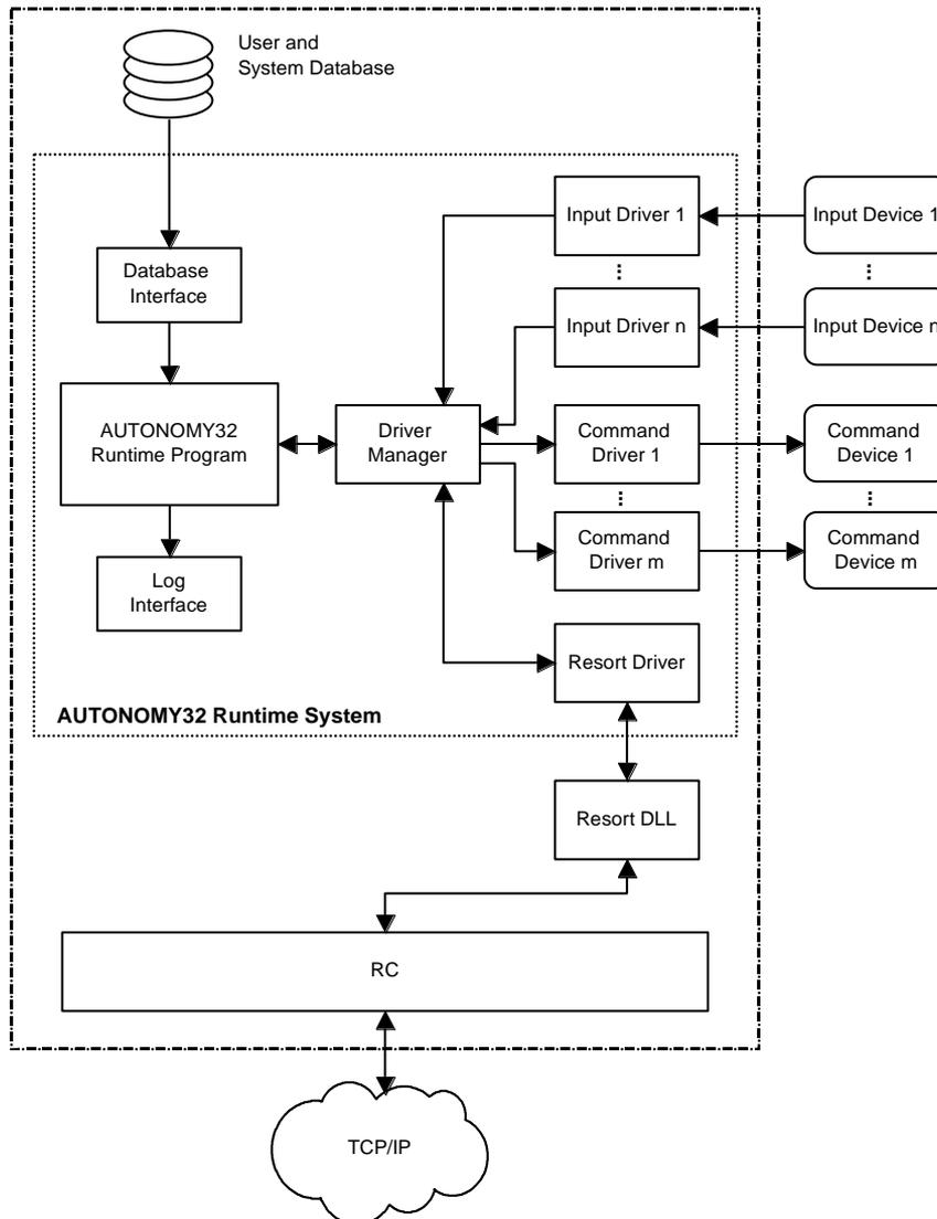
**Figure 4. The AUTONOMY system for AAC and environmental control currently is being equipped with an RCI to make it RESORTable. A local and remote RT system can be synchronised in real time even over low bandwidth channels.**
