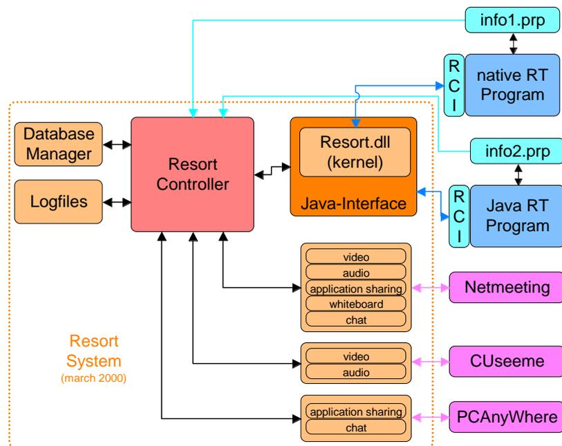
Figure 3. Internal Interfaces of the RESORT system on the local machine.
